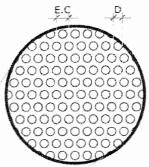
EC=13,8mm D=9,52mm DISPOSIÇÃO DOS FUROS: Alternada longitudinal
